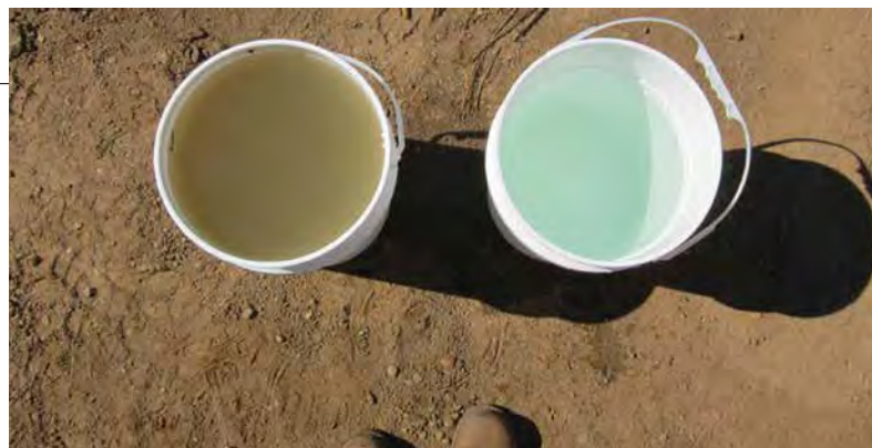
Inspired by how activated carbon removes contaminants in home water filters, Syncrude engineer Warren Zubot is now using petroleum coke—a by-product of the company’s upgrading process—to filter out contaminants in tailings water (results shown above). The rub, as always, is cost.
